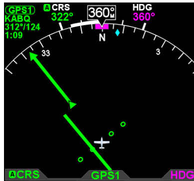
Figure 22 - ARC HSI Mode
