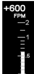
Figure 18 - Positive Rate of Climb
