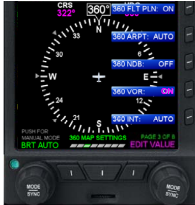
Figure 39 - Main Menu Line select keys
