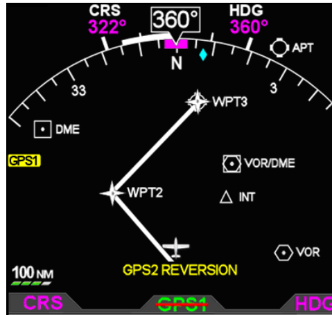
Figure 35 – GPS1 Failure, Reversionary Navigation
