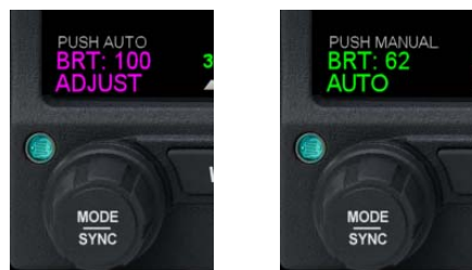
Figure 8 - Lighting control adjustment
