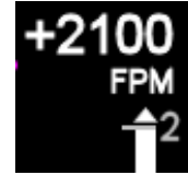
Figure 19 - Rate exceeding 2000fpm
